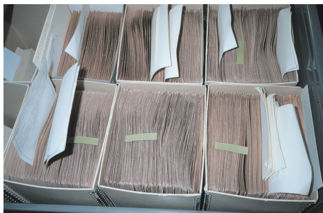
Figure 2. To test films stored in a box, place strip on top of stack and reclose box.
